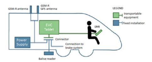
Figure 2 Schematic representation of the ETCS tablet
