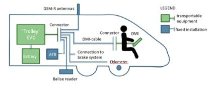
Figure 1 Schematic representation of the ETCS trolley; the battery can be a part of the fixed installation
