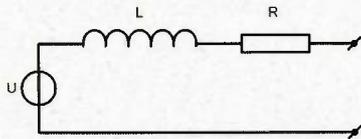
Thevenin equivalent scheme of the ATBEG antenna's with U, L and R as defined in the table above.
