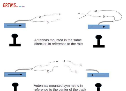
**Requirement, STMA-40589 -** The antenna + antenna installation shall not cause more than +/- 10 % tolerance (quasi constant) in the amplitude of the antenna signal due to horizontal displacements (taking into account a smallest curve (radius) of 350 m.
