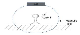
EM coupling of an antenna with the rail current.
