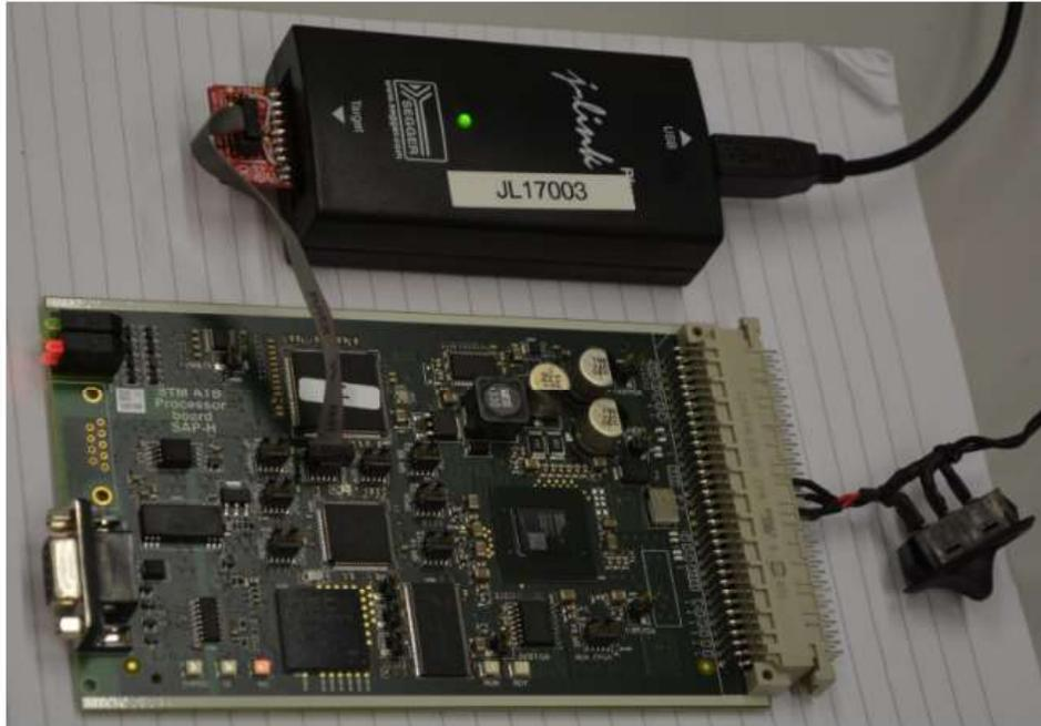
Figure 2: Hardware connections for loading the software on the Hercules processor [2219A <<vervangen>>]
