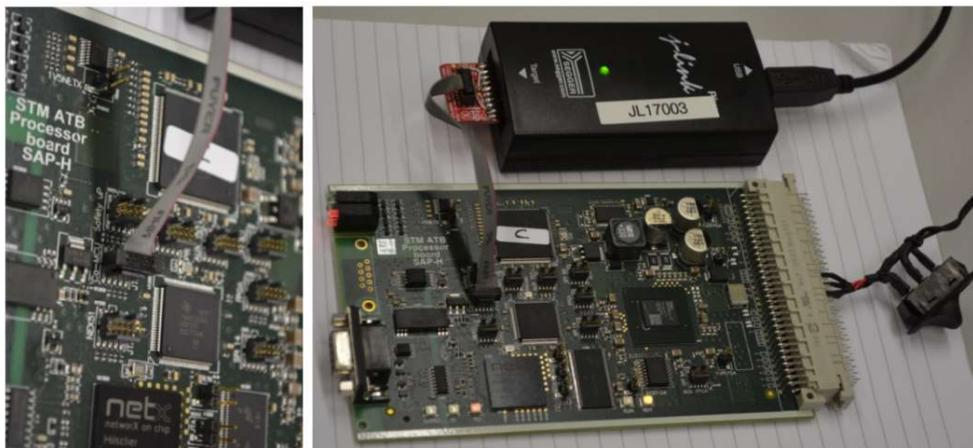
Figure 17: Hardware connections for loading the software on the TIVA co(processor) [Figure 2223A – 2226A <<vervangen>>]
