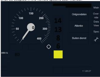
Text, STMA-75300 - After selecting driving direction forward (see the "vehicle user manual") the cab signal will be adapted according to the ATBEG code present in the track. If the cab signal is different from "Yellow" the "Gong" will sound. The "Cab Signal" shown depends on the code in the track, the speed levels related to the concerning code and the maximum speed of the train (see examples in STMA-75299 - Figure: Examples with different "Cab Signals" note: Only if the maximum speed ca... ).
