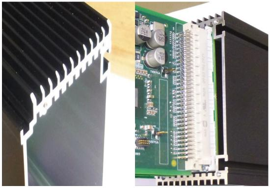
**Definition, STMA-75095 -** Slide the assembly completely into the housing until the front plate is in contact with the housing. The rear of the system should now look like the image below.
