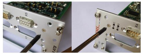
Definition, STMA-74750 - Screw the M3 SubD screws into the SubD connectors. Do not fasten them yet.
