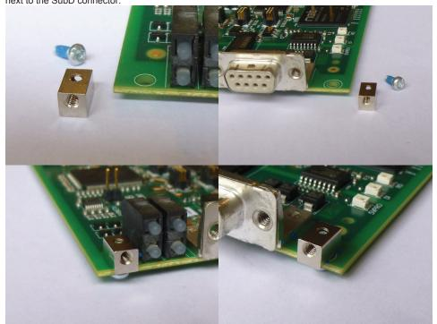
The studs are identical and have all two M3 screw holes. Position the stud in the direction as shown in the picture. The front screw hole should be oriented at the top. The stud is connected to the pcb with a screw from the underside of the PCB. Don't fasten the screws at this moment! This will allow some adjustment later on.
