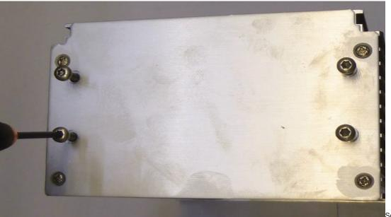
the four torx screw's (M3x10) into the inner rear panel holes into the distance blocks.
