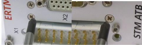
Definition, STMA-74968 - The studs must now align between the front panel and the pcb. This must be done before fastening
